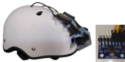
Figure 1. The Helmet with a Stereo Camera and Gyroscope Sensor MPU-6050
