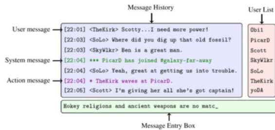
Figure 2. Abstracted chat client user interface, including examples of user, system, and action messages [5]
